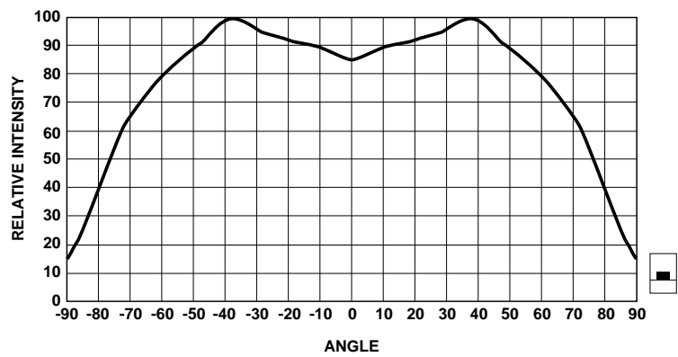
Figure 6. Relative Intensity vs. Angle for HSMx-C120.
