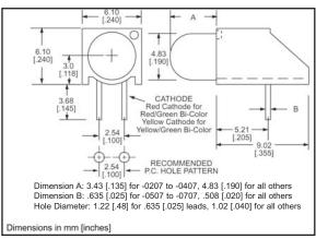
Standard Polarity shown in drawing: Cathode right
