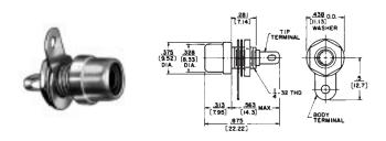
**Part Number 3501FP** 2-conductor phono jack for front-ofpanel mount, using hex nut (supplied). Only .438 inch (11.12 mm) outside dimension, can be mounted on .5 inch (12.7 mm) centers. Has 1/4 -32 bushing, mounts in .281 inch (7.14 mm) diameter hole in panels up to .25 inch (6.35 mm) thick. **INSULATED MOUNT:** Use Numbers S2207 and S1564 insulating washers (not supplied) with .313 inch (7.92 mm) diameter mounting hole. Order washers separately.
