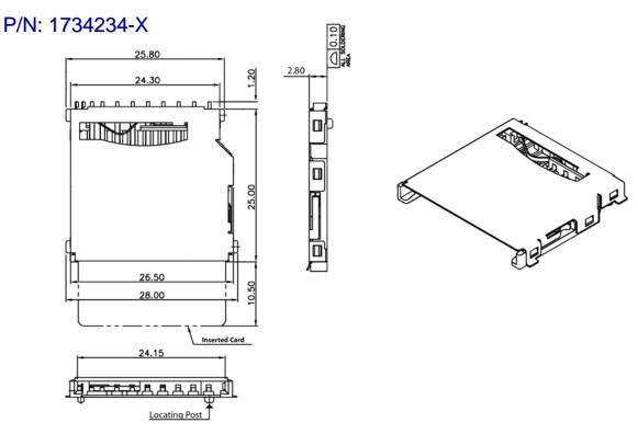
Full Size Connector: Top Mount, Push/Push Insertion/Removal
