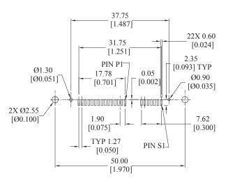
RECOMMENDED PCB LAYOUT TOLERANCE: ± 0.05 [0.002]
