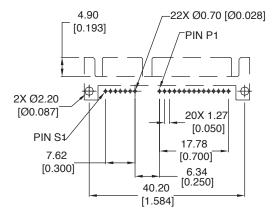
RECOMMENDED P.C.B. HOLE LAYOUT TOLERANCE ±0.05 [0.002] TOP VIEW
