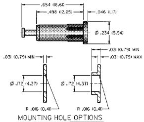
For Standard Tip Plug: .080 (2.00) Diameter FEATURES:
