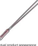
120 Series, mini glass probe, 1,000 Ohm resistance,  $\pm$ 20.0% tolerance, 25/85 BETA = 3518
