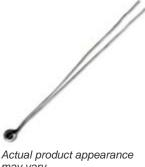
192 Series, Uni-Curve with bare leads and epoxy, 10,000 Ohm resistance, ±0,5 °C [0.9 °F] tolerance, 25/85 BETA = 3974
