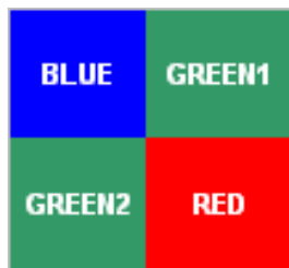
Figure 4. Color Filter Arrangement on the Pixels
