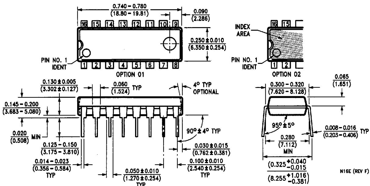
**20 Lead (0.300" Wide) Molded Dual-in-Line Package
