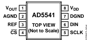
Figure 4. AD5541 Pin Configuration
