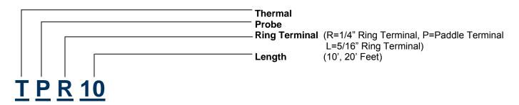
Temperature probes are available in two styles, ring terminal and paddle, and in two lengths, 10' and 20'.
