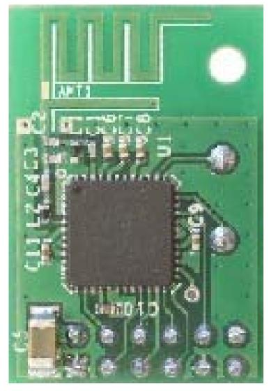
The CY3632M WirelessUSB(TM) modules are only targeted for use with the CY3632 WirelessUSB development kit, and are different from CYWM6934, which are Cypress's production-ready WirelessUSB LS(TM) modules.
