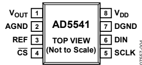
Figure 4. AD5541 Pin Configuration
