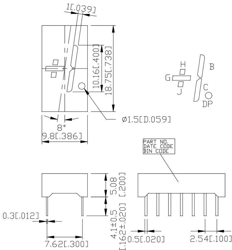
NOTES: All dimensions are in millimeters. Tolerance is  $\pm 0.25$ -mm (0.01") unless otherwise noted.
