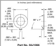
Cut round hole for the bushing and for the non-turn tab. Washer fits the double D bushing flats. Washer is sold only when accompanied by an order for a like number of switches. Washer is 302 stainless steel.
