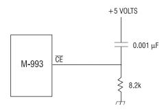
A typical control sequence for the M-993 is: (1) set data lines Selection for data settings for a particular tone pair output).to desired frequency selection, (2) wait for data lines to settle, (3) drive the chip enable (CE) low, (4) maintain CE low for desired tone duration (Note: data lines may be changed after data hold time), and (5) return CE to a logic high.
