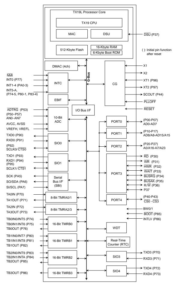
Figure 1.1 TMP1940FDBF Block Diagram
