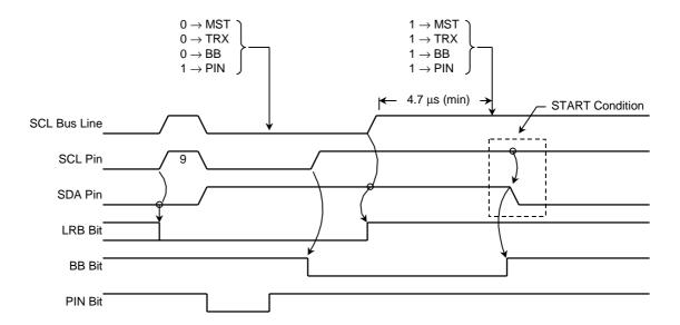
Figure 14.18 Repeated START Condition
