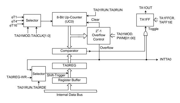
Figure 11.16 Functional Diagram of 8-Bit PWM Generation Mode
