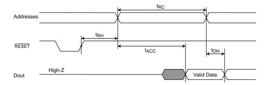
Figure 4.7 Read Timings After RESET
