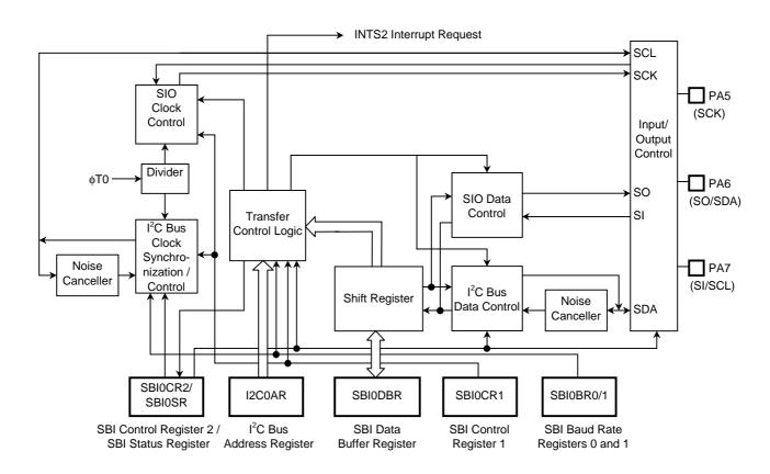
Figure 14.1 SBI Block Diagram
