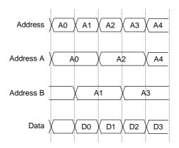
Figure 3.5 Interleave Mode
