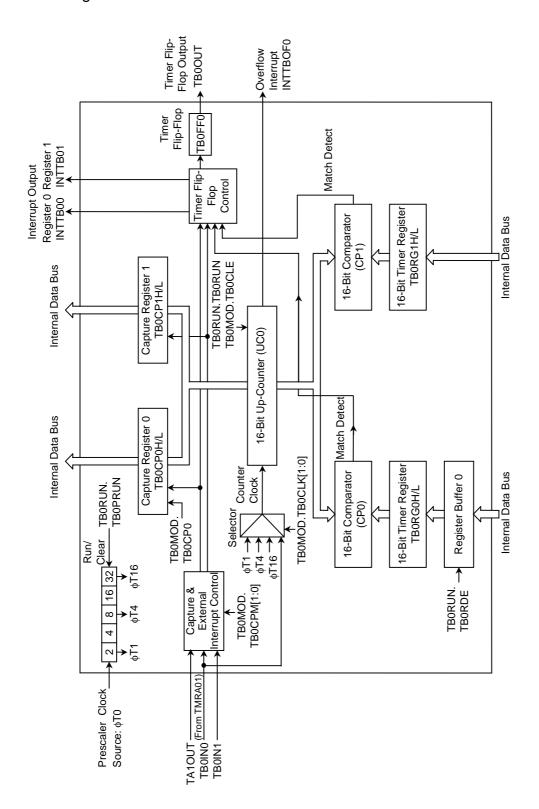
Figure 12.1 TMRB0 Block Diagram
