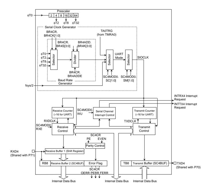
Figure 13.5 SIO4 Block Diagram
