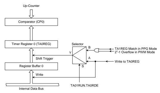
Figure 11.3 Timer Register 0 (TA0REG) Structure
