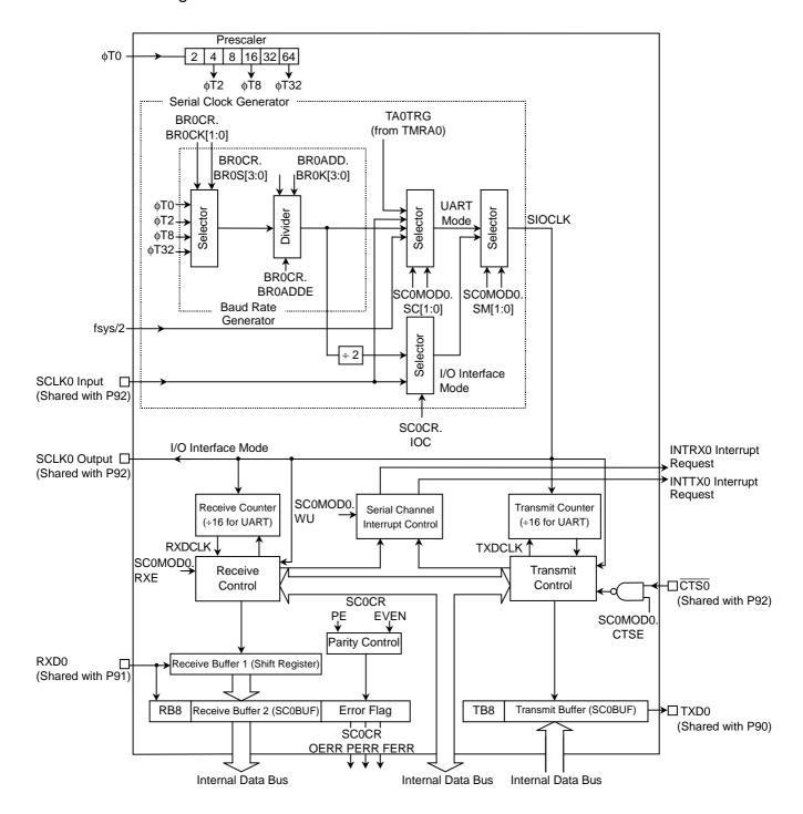
Figure 13.2 SIO0 Block Diagram
