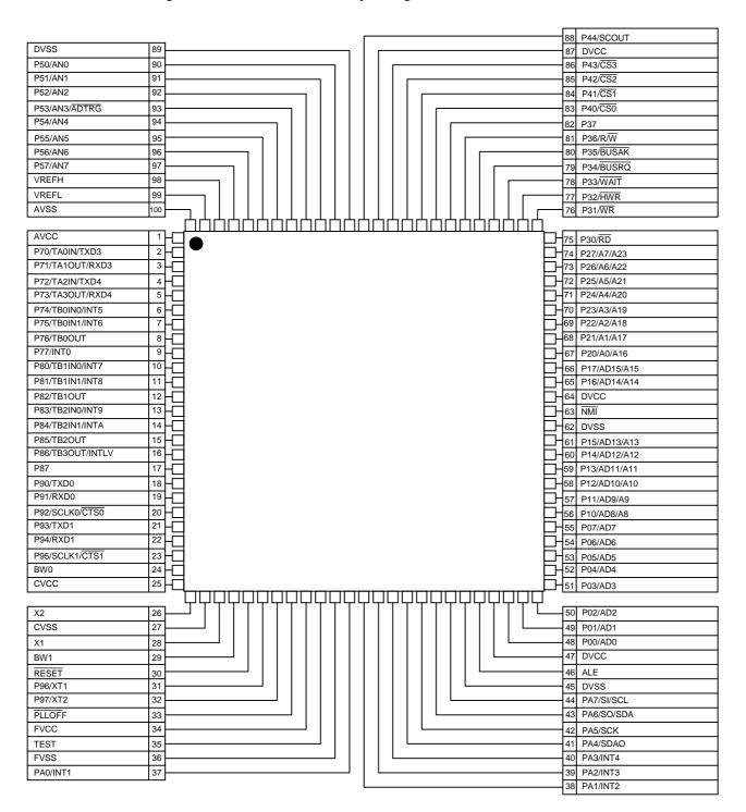
Figure 2.1 100-Pin LQFP Pin Assignment
