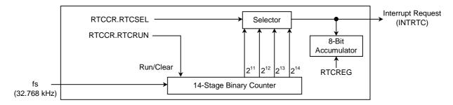
Figure 17.1 RTC Block Diagram
