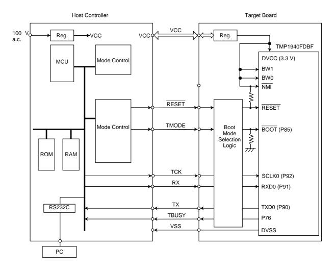
Figure 3.8 Example of a Connection Between a Host Controller and a Target Board (When the SIO0 is Configured for I/O Interface Mode)
