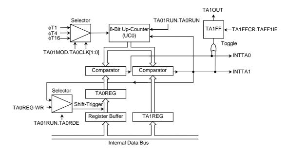
Figure 11.13 Functional Diagram of 8-Bit PPG Mode
