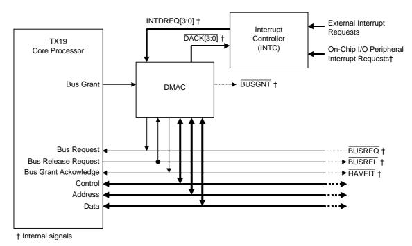
Figure 10.1 DMAC Connections within the TMP1940CYAF
