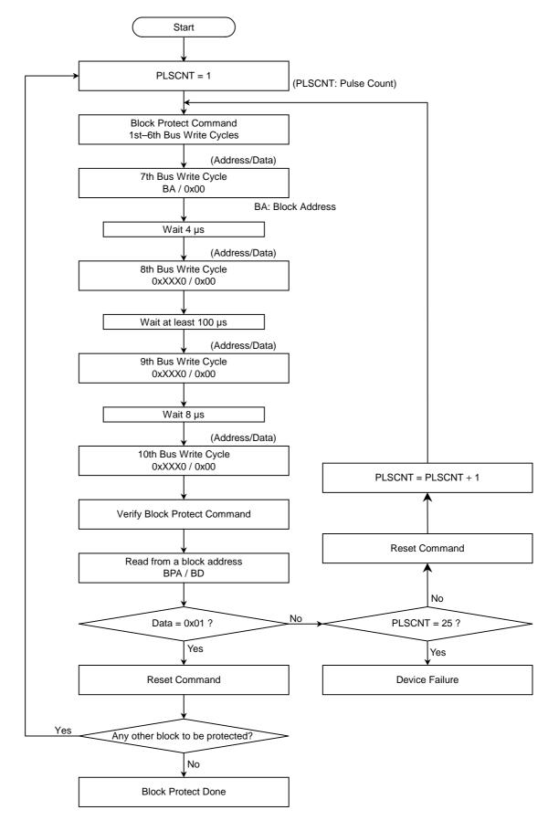
Figure 3.22 Block Protect Operation
