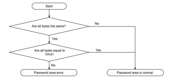
Figure 3.14 Password Area Check Flow
