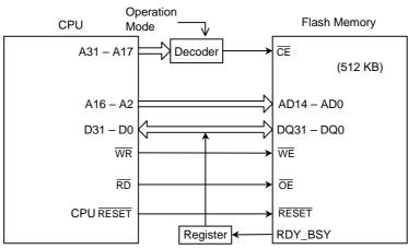
Figure 3.17 Internal CPU-to-Flash Interface
