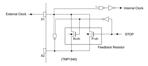
To operate the TMP1940 from an external clock, connect the clock source to the X1 pin, as shown above.
