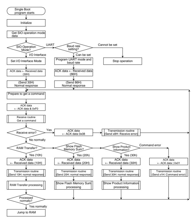
Figure 3.15 Overall Boot Program Flow
