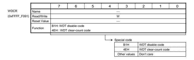
Figure 16.5 Watchdog Timer Control Register (WDCR)
