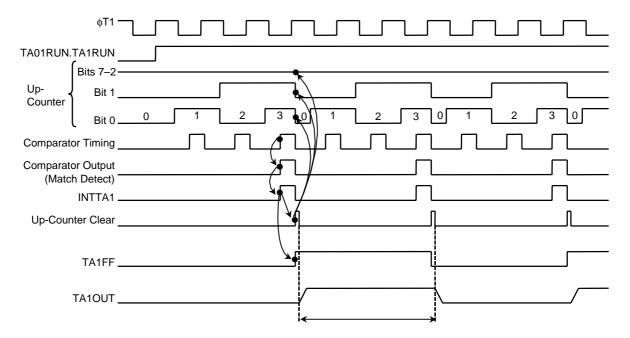
Figure 11.9 Square-Wave Generation (50% Duty Cycle)
