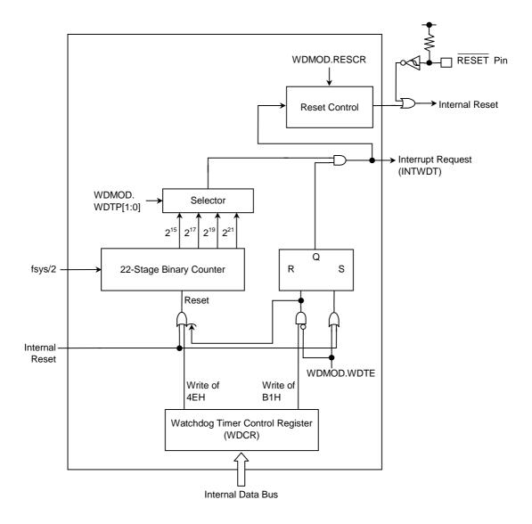
Figure 16.1 WDT Block Diagram
