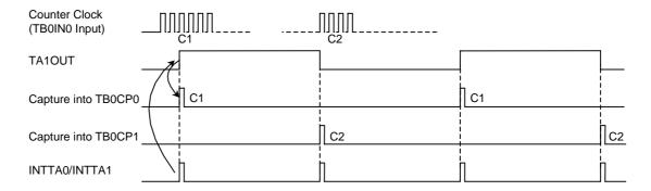
Figure 12.20 Frequency Measurement
