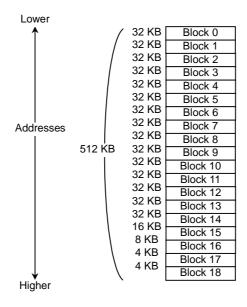
Figure 3.4 Flash Memory Block Architecture
