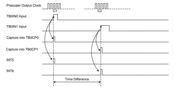
Figure 12.22 Time Difference Measurement
