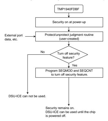
Figure 3.6 Using the Security Feature
