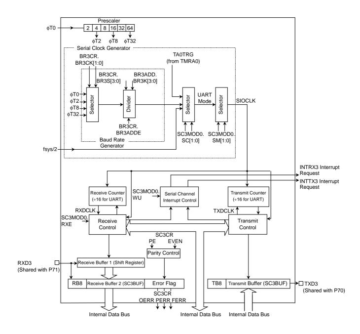
Figure 13.4 SIO3 Block Diagram
