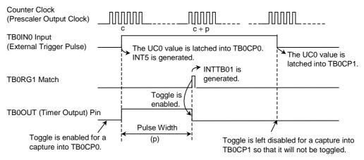
Figure 12.19 One-Shot Pulse Generation (without a Delay)
