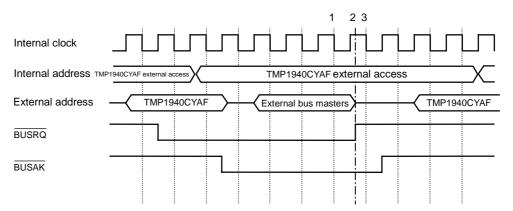
Figure 8.12 External Bus Master Relinquishing the Bus
