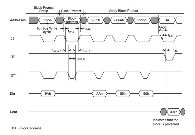
Figure 4.8 Block Protect Timings
