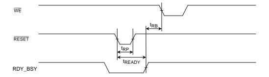
Figure 4.6 Hardware Reset Timings
