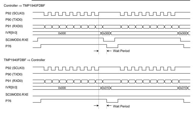
Figure 3.10 Handshake Protocol in I/O Interface Mode
