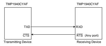
Figure 13.7 Handshaking Signals
