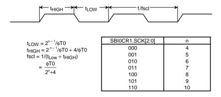
Figure 14.7 I<sup>2</sup>C Bus Clock Source
