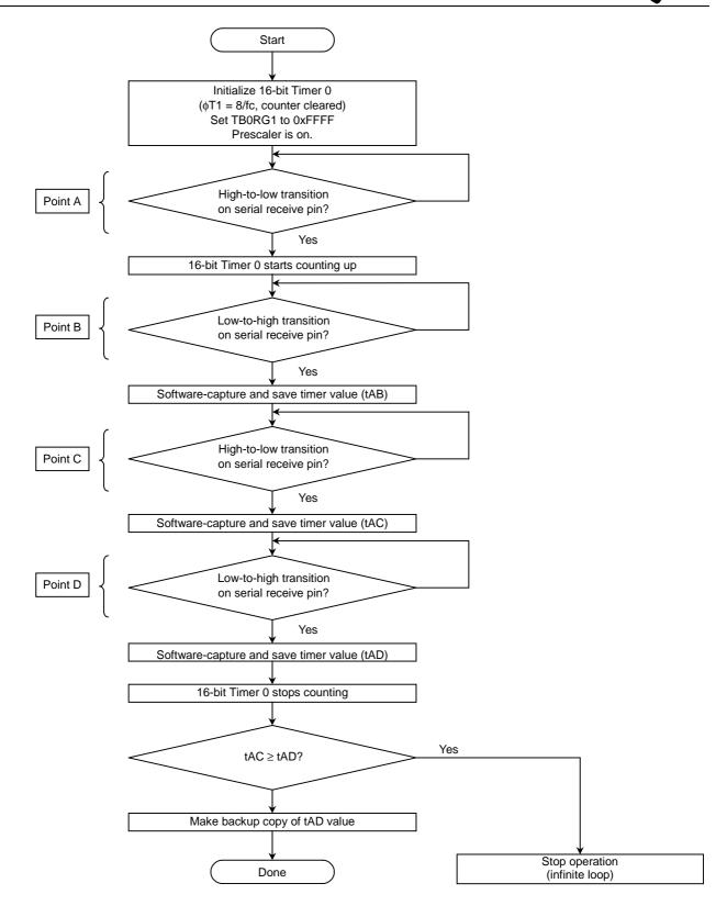
Figure 3.12 Serial Operation Mode Byte Reception Flow
