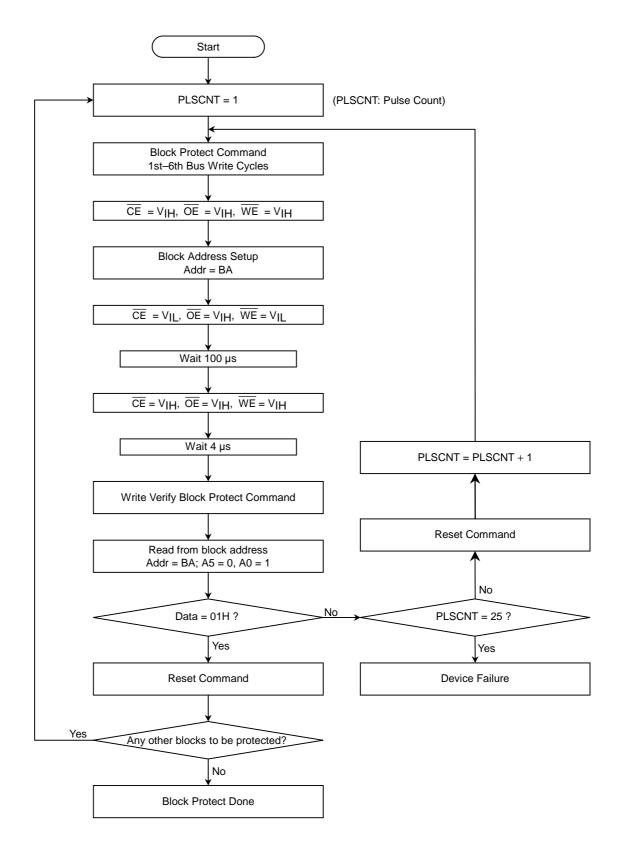
Figure 3.31 Block Protect Operation
