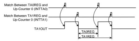
Figure 11.12 8-Bit PPG Output Waveform
