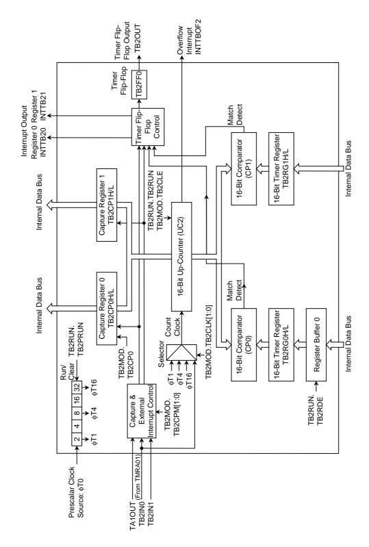
Figure 12.3 TMRB2 Block Diagram
