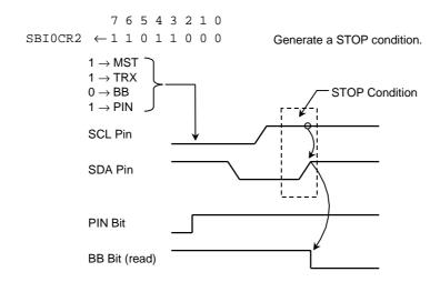
Figure 14.17 Generating a STOP Condition
