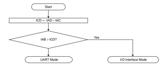
Figure 3.13 Serial Operation Mode Determination Flow
