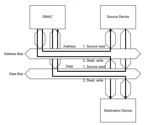
Figure 10.12 Dual-Address Transfer Mode
