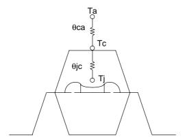
Figure 2 Thermal resistance of package
