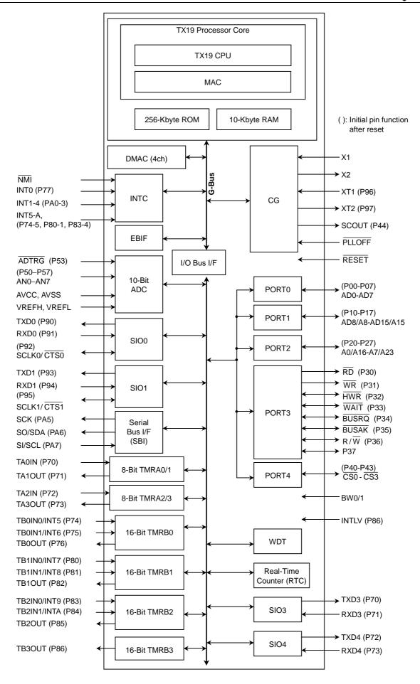
Figure 1.1 TMP1940CYAF Block Diagram
