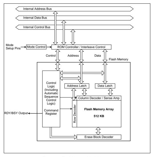
Figure 3.1 Flash Memory Block Diagram
