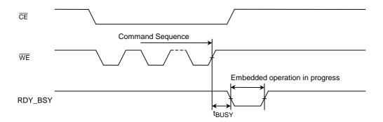
Figure 4.5 RDY\_BSY Status Timings During Embedded Operations
