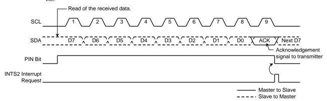
Figure 14.15 SBI0CR1.BC[2:0] = 000 and SBI0CR1.ACK = 1 (Master-Receiver Mode)
