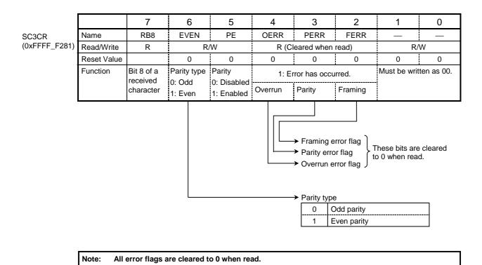
Figure 13.15 SIO3 Control Register (SC3CR)
