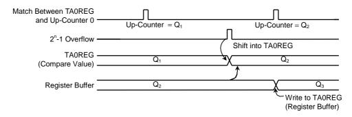
Figure 11.17 Register Buffer Operation
