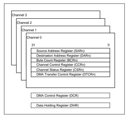
Figure 10.2 DMAC Block Diagram
