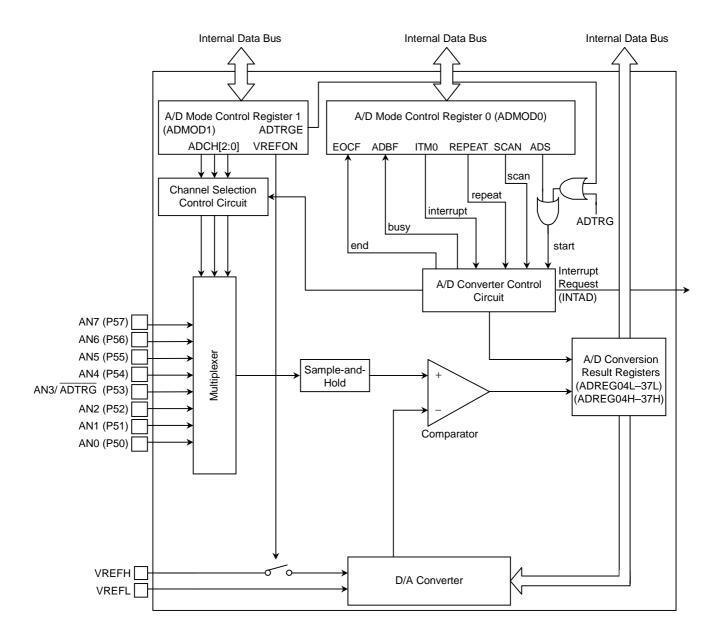
Figure 15.1 ADC Block Diagram
