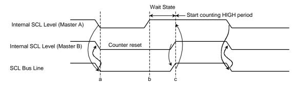
Figure 14.8 Clock Synchronization Example
