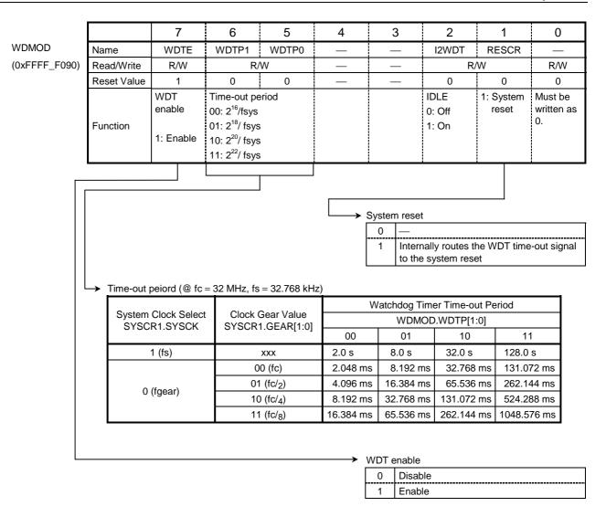
Figure 16.4 Watchdog Timer Mode Register (WDMOD)
