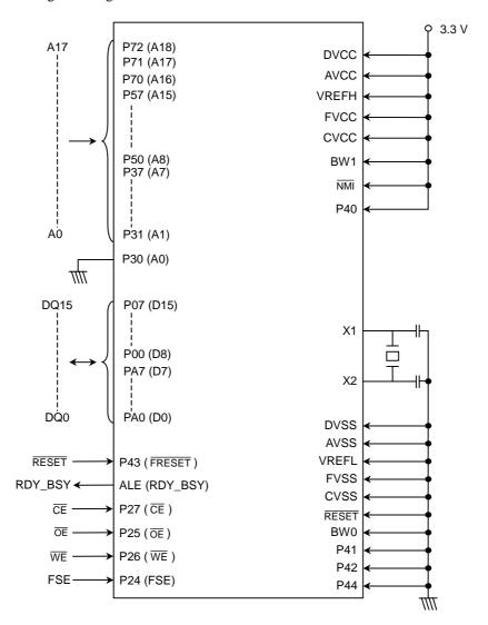
Figure 3.25 Pin Settings for Programmer Mode
