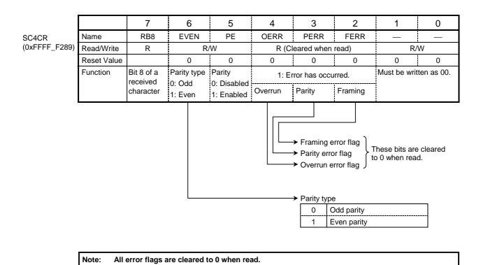
Figure 13.16 SIO4 Control Register (SC4CR)
