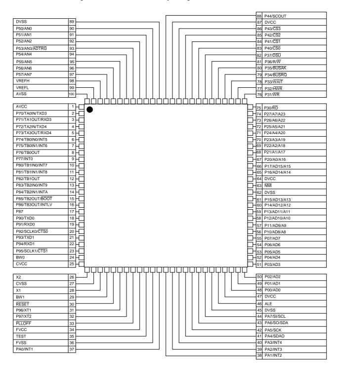
Figure 2.1 100-Pin LQFP Pin Assignment
