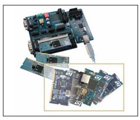
including the REva evaluation board, microcontrollers, embedded RLink JTAG in-circuit debugger/programmer and Raisonance Integrated Development Environment (RIDE).
