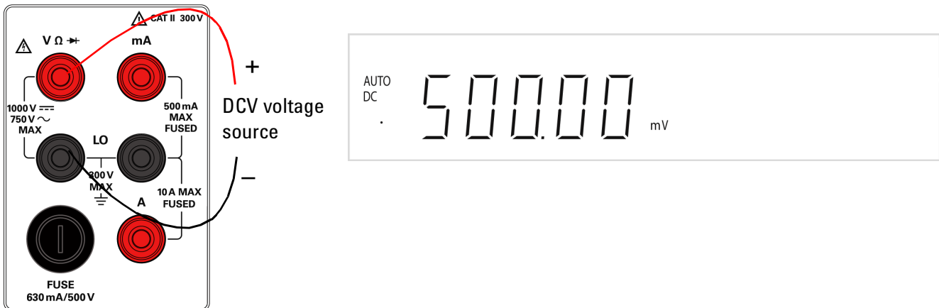
Figure 2-2 DCV terminal connection and display
