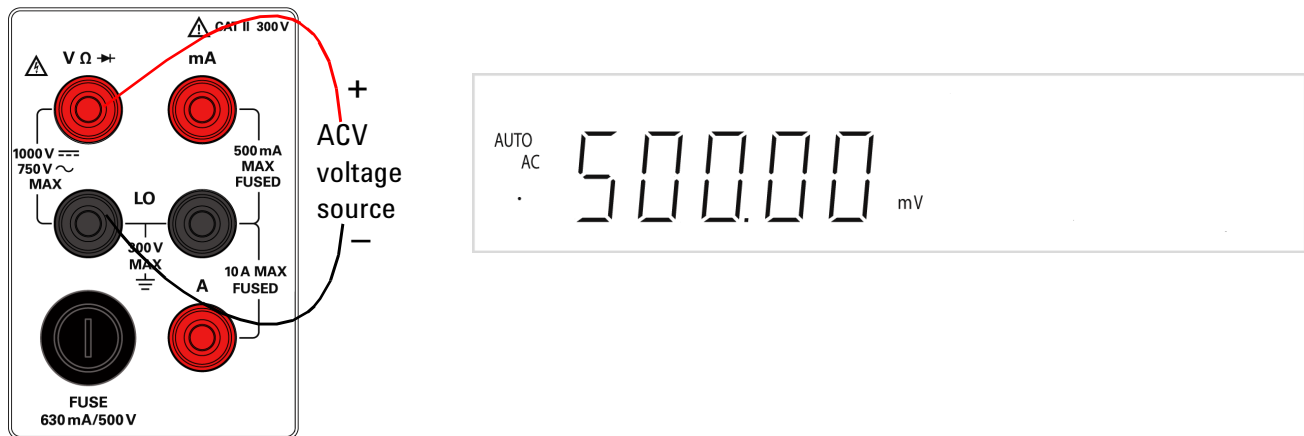
Figure 2-1 ACV terminal connection and display
