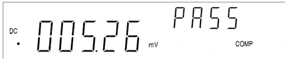
Figure 2-14 Typical Comp operation display
