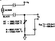
For most applications, a single point calibration is sufficient. With the probe at a known temperature, adjust  $R_{T}$  so that  $V_{O}$  corresponds to the known
