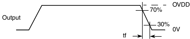
Figure 7. Definition of Timing for Standard and Fast-Mode
