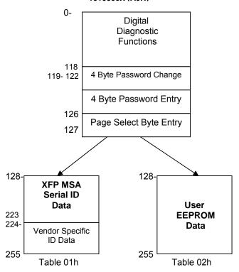
The Transceiver module provides a lower memory (byte address 0-127) as well as table 01h and table 02h. The device address of module is always A0h.
