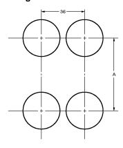
The pitch A, between the centers of the mounting holes, is shown below.
