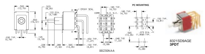
Not available with JXX actuators and I seal option. Terminal bend radii and lead-in manufacturing option.
