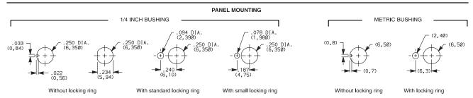
**NOTE:** Two mounting nuts, locking ring and lockwasher supplied standard with threaded bushings. Optional mounting nut and locking ring styles available, see section "Technical Data and Additional Hardware".
