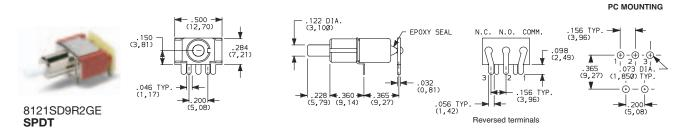
Not available with JXX actuators, D3, H, H9, Y3, Y4 bushings, I seal option.
