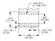
SHORT PCB, TYPE 0 WITH SOLDER PINS
