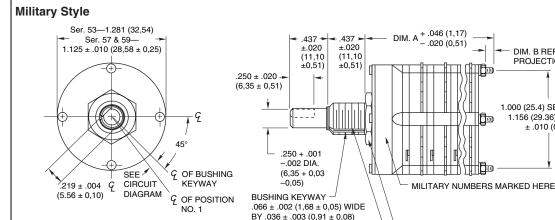
BY .036 ± .003 (0,91 ± 0,08) DEEP FROM A .375 (9,53) DIA. INTEGRAL ASSEMBLY NUT. DO NOT REMOVE. 3/8-32 UNEF-2A THREAD
