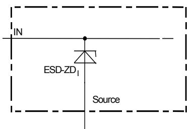
ESD zener diodes are not designed for DC current > 2 mA @  $V_{IN} > 10V$ .
