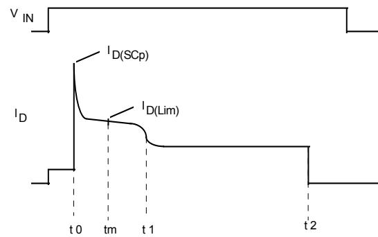
$t_0$ : Turn on into a short circuit
