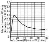
RELATIVE LUMINOUS EFFICIENCY (LUMINOUS INTENSITY PER UNIT CURRENT) VS. PEAK CURRENT (REFRESH RATE 1KHz)
