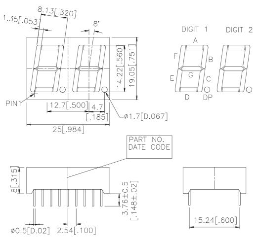
NOTES: All dimensions are in millimeters. Tolerances are ± 0.25 mm (0.01") unless otherwise noted.
