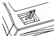
Figure 8: Master Setting for Vertical iDiskOnChip 44-Pin Connector
