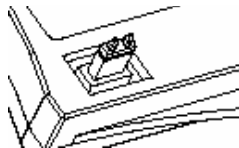
Figure 6: Slave Setting for Vertical iDiskOnChip 44-Pin Connector
