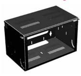
Hinged panel pivots to 90 degrees with positive stop, providing a stable platform for punch-down interconnects. Thumbscrews secure the panel in the upright position. Integral VELCRO® cable tiedown slots facilitate cable routing. Cover protects equipment and cables. Made of 12 gauge steel on hinged swing-out frame; 16 gauge on body. Finished with RAL 9005 low gloss black polyester powder paint. Shipped fully assembled.
