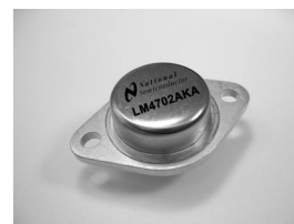
Metal Can — 15 Lead TO-3 (for LM4702A, in development)
