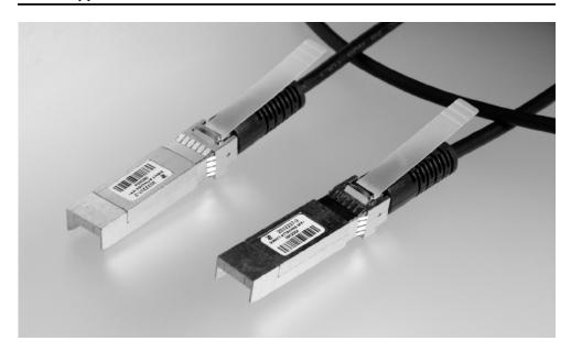
The Tyco Electronics SFP+ direct attach copper cable assembly is a low cost alternative for short reach applications. The design allows for a serial data transmission up to 10 Gbps in each direction. These SFP+ assemblies are hot swappable and the programmed EEPROM
