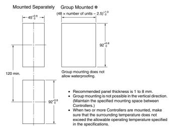
\* Group mounting is not possible if an SSR output is used for control output 1 or 2 and the E53-C3N or E53-C3DN Output Unit is used. For these combinations, maintain the following mounting space between Controllers.
