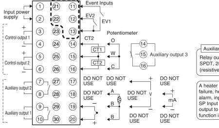
Auxiliary output 3 Relay output SPDT, 250 VAC, 3 A (resistive load)
