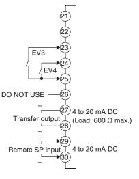
Note: Wire all voltage input terminals correctly. The Controller may fail if voltage input terminals are wired incorrectly.
