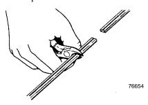
3.02 Slit drop wire approximately 1 1/4" (32 mm) with a drop wire splitter.
