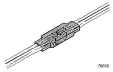
3.04 Important: Press both thumbs down equally on the connector cap. You will hear a "crunch." This means the connector is pre-crimped. (This will help hold the drop wires in place until the connector is crimped).
