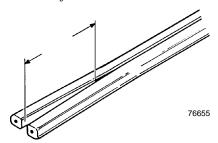
3.03 Line up ribs of drop wires so that tip and ring are not reversed at the splice. Slide one of the drop wires into the connector. Holding connector and drop wire, insert the other drop wire. Make sure both drop wires are inserted all the way.
