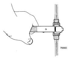
3.07 When connector is used midspan, provide additional strain relief by using two drop wire clamps. Make sure that the clamps are locked onto the drop wires by tapping the clamps to set the teeth.
