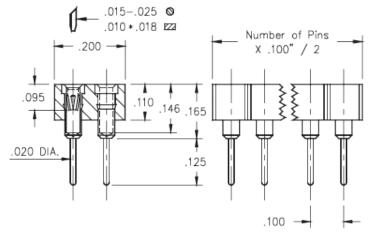
**Description:** Interconnect Socket .100 Grid; Straight Socket Standard Solder Tail (0.125 Tail) Double Row Through Hole Accepts .015-.025" Leads Plating Code:
