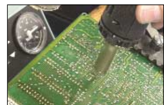
Through hole rework with the DSV80
