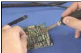
The PES51 can handle most general purpose hand soldering applications.
