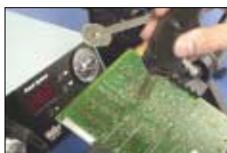
DSV80 in-line desoldering tool with internal solder collection chamber
