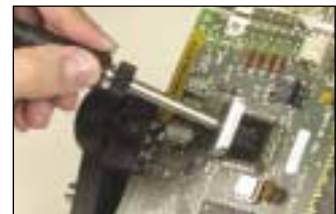
A SMT quad tip is used to desolder a quad flat pack.
