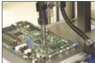
Step 2: The nozzle is lowered onto the component to effect reflow and engage the component to the vacuum pick-up.
