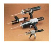
simultaneously meter, mix and apply twopart adhesives and potting compounds. System features handy 3M™ Scotch-Weld™ Duo-Pak Adhesive Cartridges that snap quickly into the durable, lightweight EPX applicator. A slight squeeze on the trigger advances the plunger into the cartridge. Accurate measurement and the mixing nozzle provides thorough mixing and precise placement of material. Ideal system for assembly, maintenance and in-field service.
