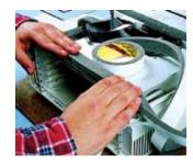
conformable low density urethane foam which can help seal out air, dust, and light when compressed 50%. Vinyl foam tape series 4500 and 4700 are durable, flexible closed cell vinyls which can help seal out dust, light, and moisture when placed under 30% compression. All foams feature an acrylic adhesive. 3.0 mm thickness.
