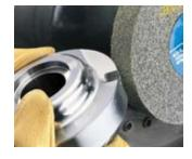
of loose-flying wires. Maximum RPM: 12,100. Use Mandrel No. 990. Gray/Black.
