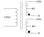
\* Secondary windings are designed to be connected in series or parallel. Windings are not intended to be used independently.
