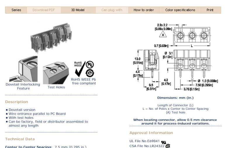
Center to Center Spacing: 7.5 mm (0.295 in.) Nominal Cross Section: 2.5 mm<sup>2</sup> (3874 mils<sup>2</sup>) Wire Stripping Length: 7 mm (0.28 in.) Recommended Hole Diameter in PC Board: 1.3 mm (0.051 in.)
