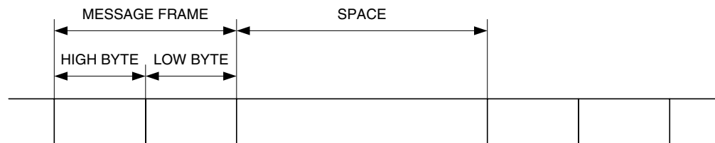
Figure 3-5. Message Frame and Space
