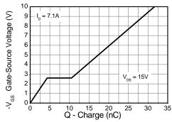
Gate-Source Voltage v Gate Charge
