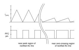
Figure 13: On-time modulation circuit timing diagram
