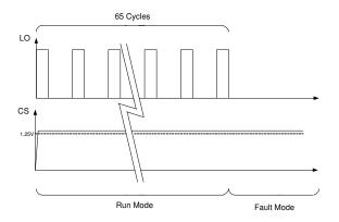
Figure 3: Fault counter timing diagram.
