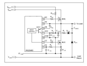
Figure 1: Start-up and supply circuitry.
