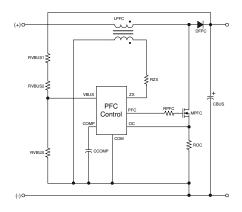
Figure 10: IRS2548D simplified PFC control circuit.
