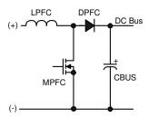
Figure 8: Boost converter circuit.
