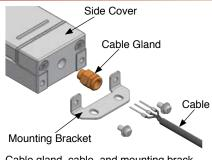
Cable gland, cable, and mounting brackets are also available as accessories for installation in various applications.
