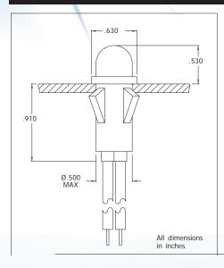
Mounting: Will snap-fit into  $\emptyset$ .500/.505 hole in panels .020/.100 thick. Push-on speednut SN0461 also available.
