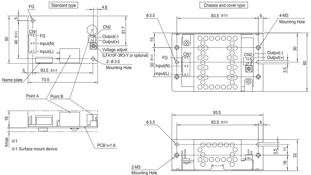
※ The back side of P.C.B. of the power supply is assembled some SMDs.
