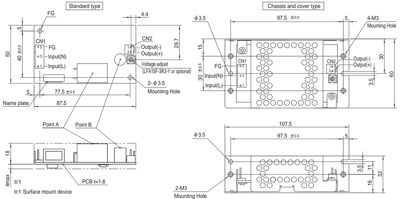
※ The back side of P.C.B. of the power supply is assembled some SMDs.
