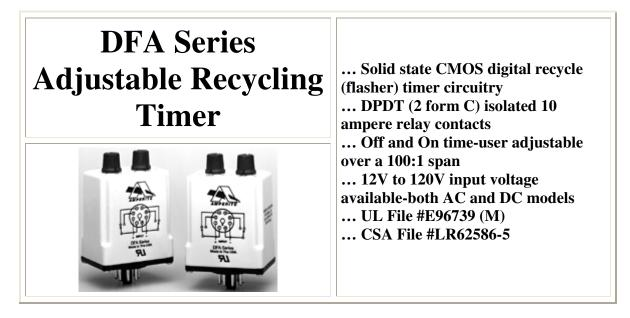
The Amperite DFA series adjustable recycling timers provide a continuously operating off/on cycle as long as power is applied to the input terminals. Two knob operated potentiometers provide user adjustment of both the flash rate and duty cycle. One knob sets the Off time; the other sets the On time. Standard models allow both the Off time and On time to be adjusted over a 100:1 range. Custom timing is available.
