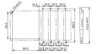
Mounting hole layout from left, FC4A-HPH1, FC4A-D20K3, FC4A-N16B3, FC4A-N32B3, and FC4A-M24BR2 modules
