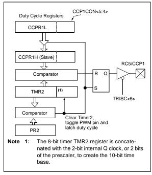
The PWM output (Figure 8-4) has a time base (period) and a time that the output stays high (duty cycle). The frequency of the PWM is the inverse of the period (1/period).
