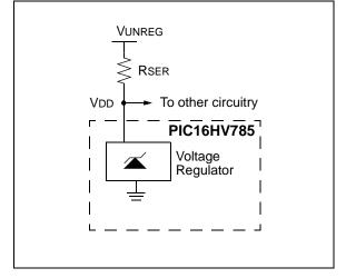
An external current limiting resistor, RSER, located between the unregulated supply, VUNREG, and the VDD pin, drops the difference in voltage between VUNREG and VDD. RSER must be between RMAX and RMIN as defined by Equation 16-1.
