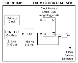
The FSCM function is enabled by setting the FCMEN bit in Configuration Word (CONFIG). It is applicable to all external clock options (LP, XT, HS, EC, RC or I/O modes).
