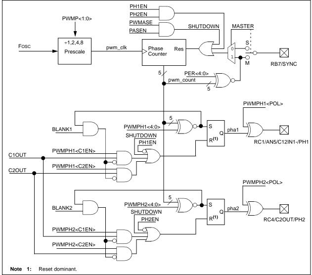
FIGURE 13-1: TWO-PHASE PWM SIMPLIFIED BLOCK DIAGRAM
