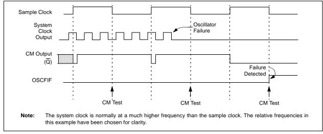
FIGURE 3-9: FSCM TIMING DIAGRAM
