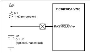
An internal MCLR option is enabled by clearing the MCLRE bit in the Configuration Word. When cleared, MCLR is internally tied to VDD and an internal Weak Pull-up is enabled for the MCLR pin. The VPP function of the RA3/MCLR/VPP pin is not affected by selecting the internal MCLR option.
