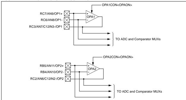
FIGURE 11-1: OPA MODULE BLOCK DIAGRAM
